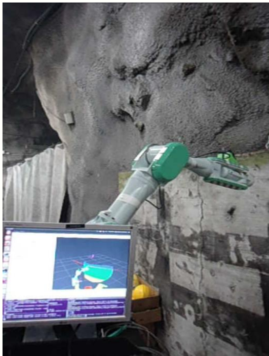
The Robotic Arm System during the VSH tests. In the monitor one can see also the scanned surface and the state of the robot
