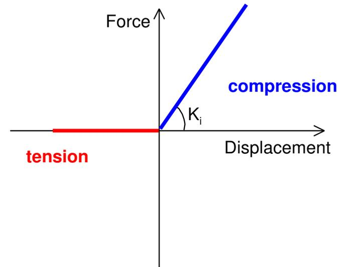
$K_i$  values =  $f(\text{rockmass, lining geometry})$
