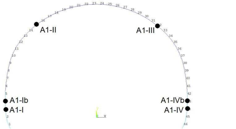
zone of high axial force requirement for low eccentricity (crack control)
